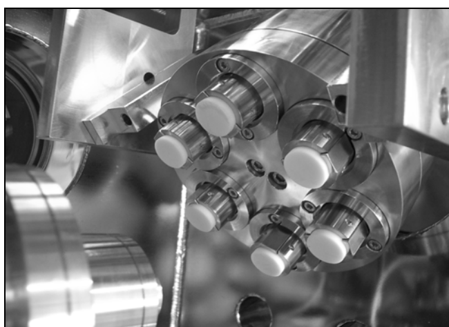
Fig.2 Target holder in an advanced PLD vacuum system, consisting of six rotatable targets.
