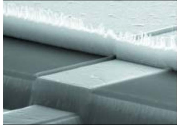
**MBE magic:** light emission from a blue laser-diode wafer grown by MBE (left) and a scanning electron microscope image of the structure showing the dry-etched laser facet (right). Sharp is now working hard to improve the laser's performance.
