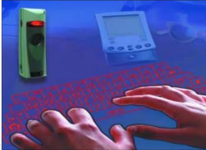
Light touch: iBIZ's Virtual Laser Keyboard makes it easier to enter data into a PDA.
