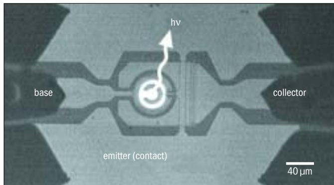
**Bridging the gap: the researchers say their light-emitting transistor is the key to high-speed signal processing involving both electrical signals and optical signals.**
