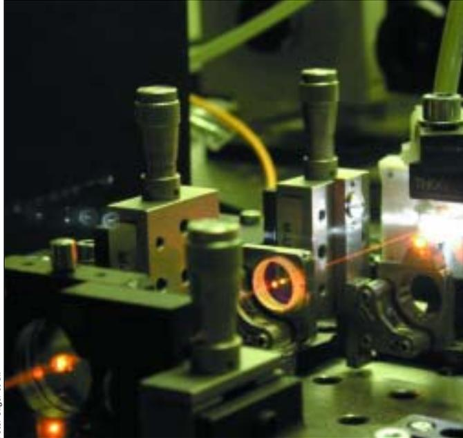
Orange emitter: the external mirror can be seen in the centre of the image and the doubling crystal on the right. The doubling crystal is hiding the semiconductor disk.
