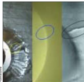
Shedding some light: from left to right, visible, dye-based fluorescence and photothermal images of a crack in a metal component. The crack is almost invisible in the first two images but shows up clearly in the third as an imperfection measuring 12 mm long.
