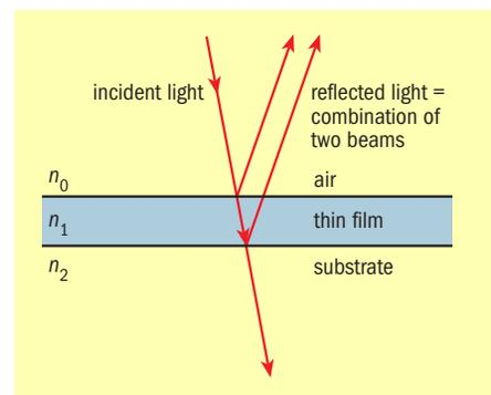
**The principle of a thin-film coating:** interference between reflections from a single film (above) or multiple layers (left) determines the precise optical characteristics of a particular coating.
