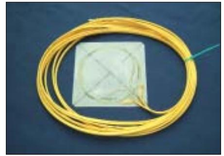
An Insensys rosette patch for measuring strain. It contains two FBGs at right angles to each other.
