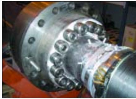
Lucrative market: optical-fibre strain sensors deployed in oil riser pipes could be big business.
