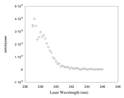
Ionisation spectrum of  $Ta_4C_4$  showing onset of ionization at 241 nm
