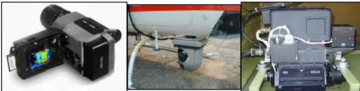
Figure 3—Hand-held infrared imager ( left ); gimbaled-mounted turret FLIR system ( middle ), and nadir-mounted line scanner ( right ).
