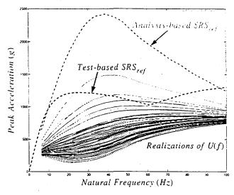
Figure 11: Analytically-based reference SRS.
