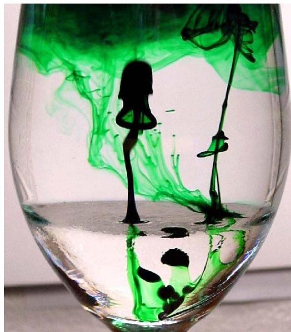
Figure 1: Buoyancy Through Interface . A buoyant jet of dyed 70% isopropyl alcohol rises through the interface formed by corn syrup and water. Jessica Todd.
