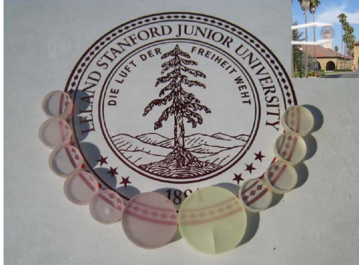
Fig.4 Pellets of Nd:YAG (left pink samples) and Gd:YAG(right yellow samples) on the sunlight.
